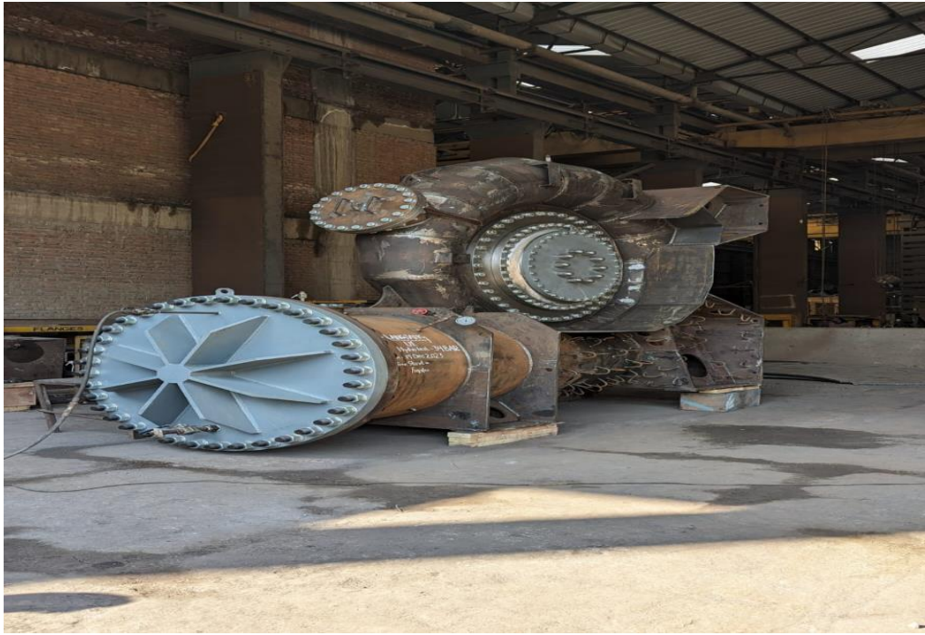
Figure: Spiral casing ready for pressure and leakage test
