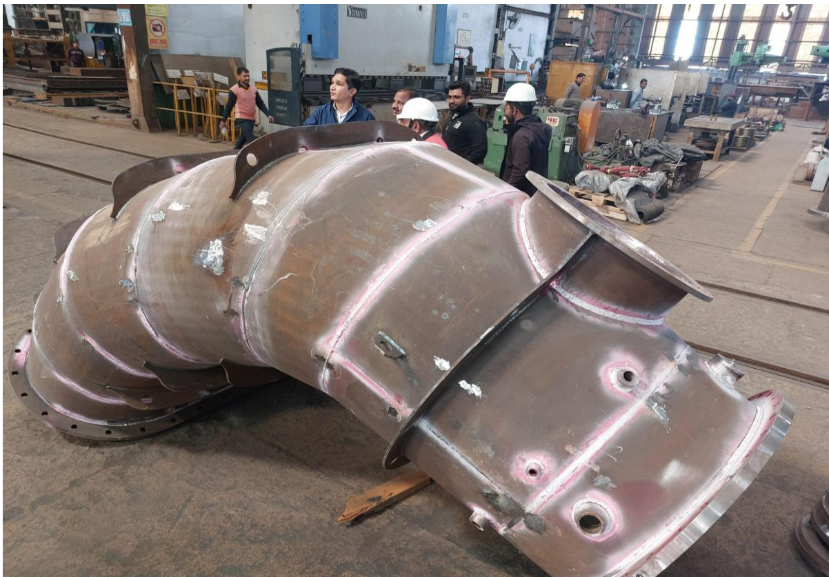
Figure: Draft tube Visual Inspection
